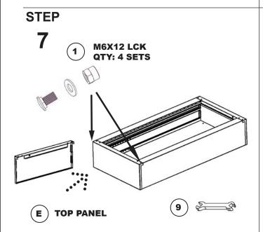
SLIDE TOP PANEL OVER THE SIDE, CENTER AND BACK PANELS. INSERT 4 - M6X12 BOLTS THROUGH FRONT AND FULLY TIGHTEN WASHER & LOCK NUTS FROM INSIDE USING WRENCH.
