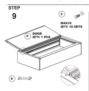
FOLD DOOR HINGE FULLY OPEN. LAY DOOR ONTO LEFT FRONT FRAME OF CABINET. LINE UP PRE-DRILLED HOLES IN HINGE AND DOOR FRAME. INSERT M4X10 THROUGH DOOR HINGE AND ATTACH NUT FROM INSIDE AND FULLY TIGHTEN USING WRENCH.
