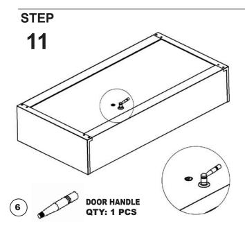
SCREW LOCK HANDLE INTO DOOR. OPEN AND CLOSE DOOR TO CONFIRM PROPER ALIGNMENT.
