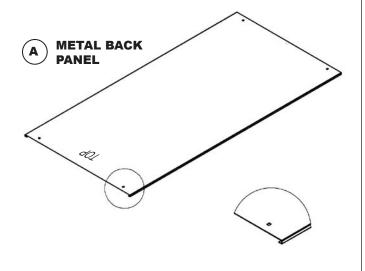
LAY METAL BACK PANEL ON FLOOR WITH INSIDE OF BACK PANEL FACING UP.
