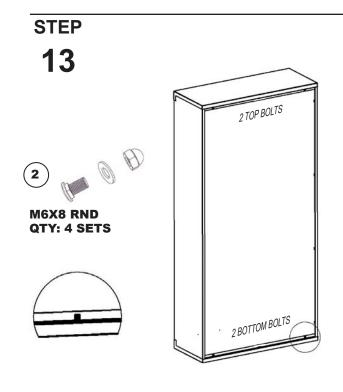
INSERT 4 - M6X8 RND BOLTS THROUGH BACK AND FULLY TIGHTEN WASHER & ROUND HEADED LOCK NUTS FROM INSIDE USING M6 WRENCH.
