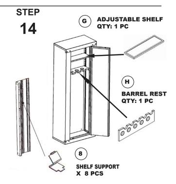
INSERT METAL STORAGE SHELVE AND BARREL REST IN THE CABINET USING SHELF SUPPORTS IN THE DESIRED LOCATION.
