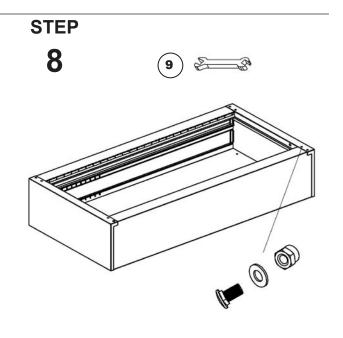
RETURN TO BOTTOM PANEL AND FULLY TIGHTEN THE 4 - M6X12 BOLTS FROM INSIDE USING THE WRENCH.
